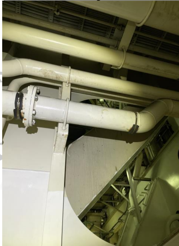
Pictures of other deficiency: Section of insulation missing on the turbocharger exhaust pipe of all 4 generators
