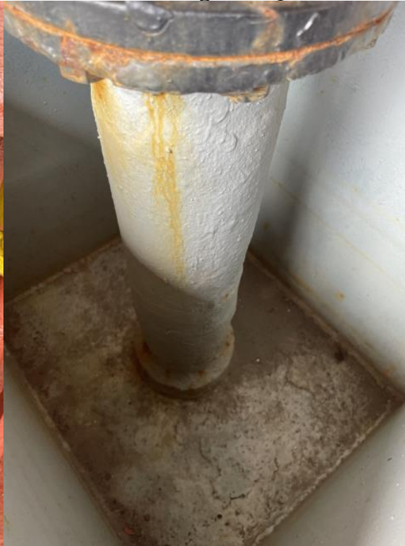
Pictures of other deficiency: Air pipe of HFO tank no. 4P forward and HFO no. 5P forward temporarily repaired with canvas bandage and painted.
