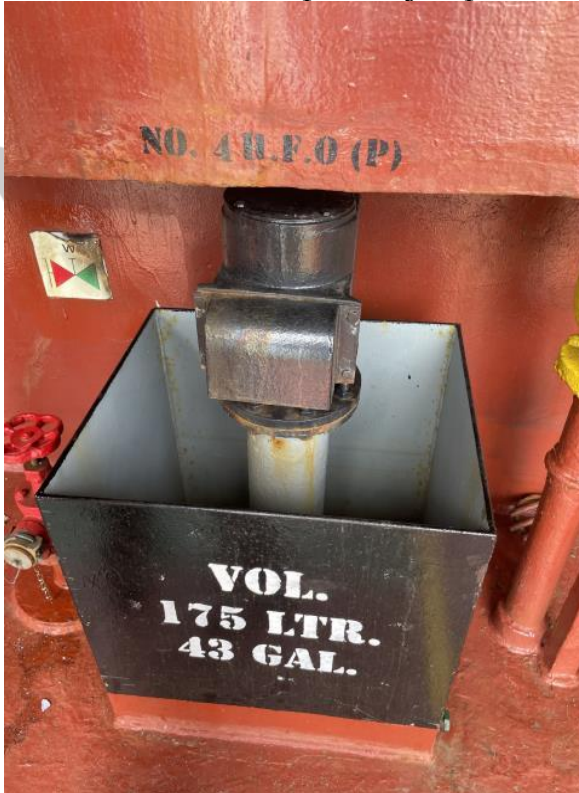
Pictures of other deficiency: Air pipe of HFO tank no. 4P forward and HFO no. 5P forward temporarily repaired with canvas bandage and painted.
